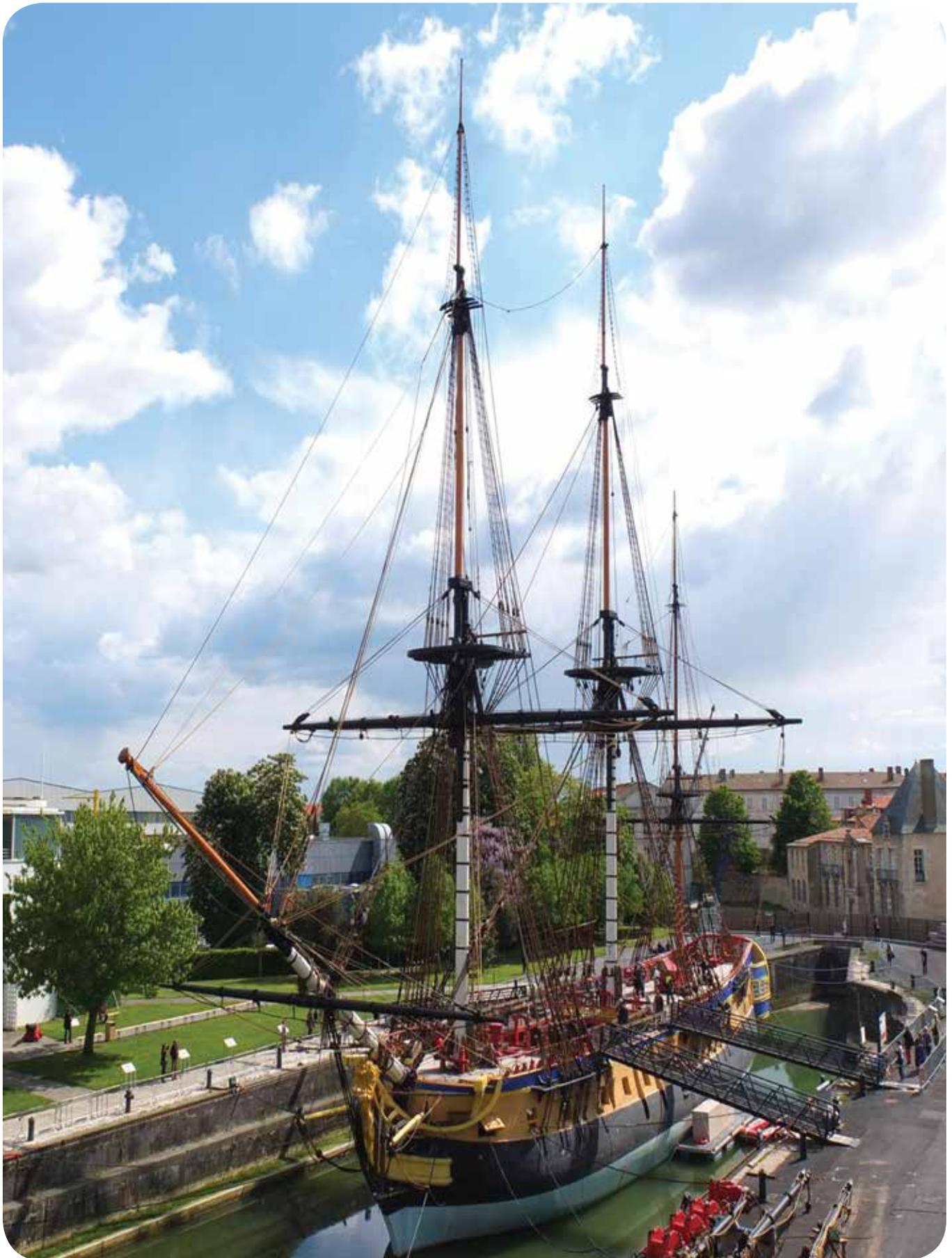
**Photo 5.** With her launch and masting completed, the new *Hermione* awaits her topsail and topgallant yards and completion of her rigging, in the Spring of 2013.
