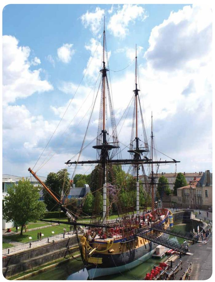
**Photo 5.** With her launch and masting completed, the new *Hermione* awaits her topsail and topgallant yards and completion of her rigging, in the Spring of 2013.
